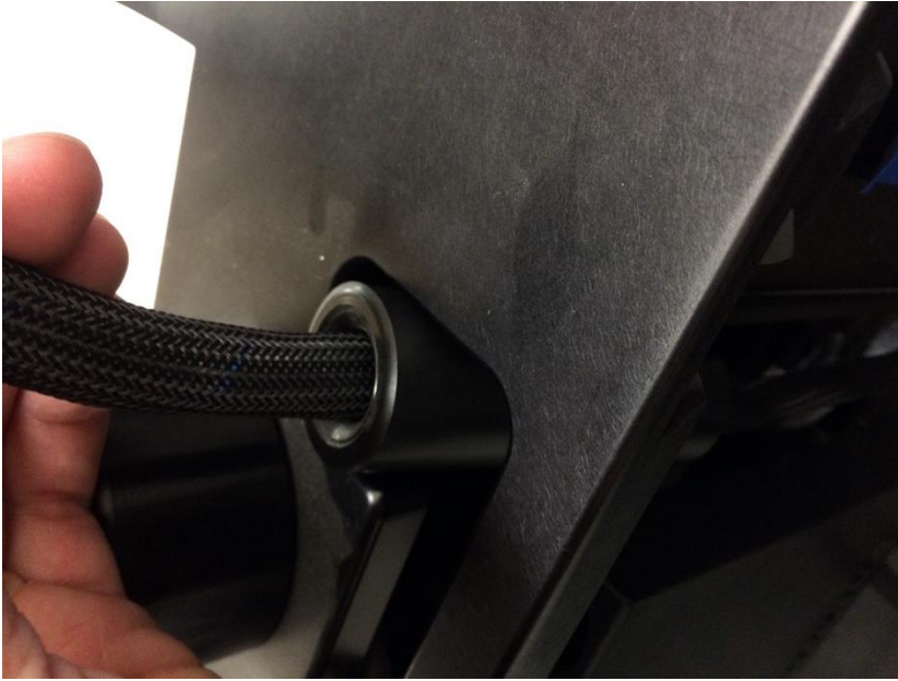
Connect Colordome to Colordome Power Supply
