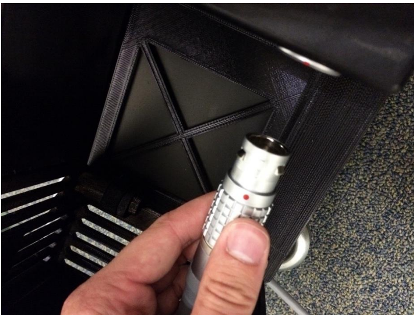
Connect Colordome coax video cable to Video in coax connector located on the Colordome Power Supply. Use USB B to USB A cable to connect USB video out on CD Power Supply to USB port of Computer.
