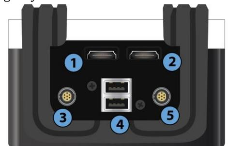
Figure 3 - Celeris connections, left front panel
