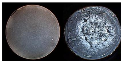
Figure 42 - Closeups of clean (left) and dirty (right) full-field electrodes
