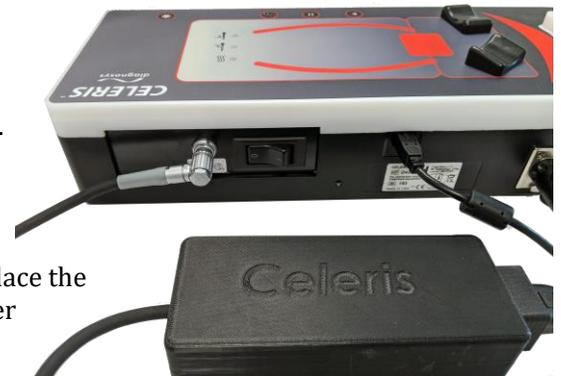
Figure 2 - Celeris Power Supply & connection to console
