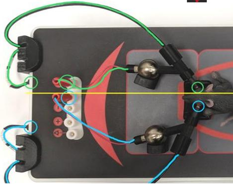
Figure 15 - Amplifier Setup of a *TOUCH/TOUCH™* Protocol
