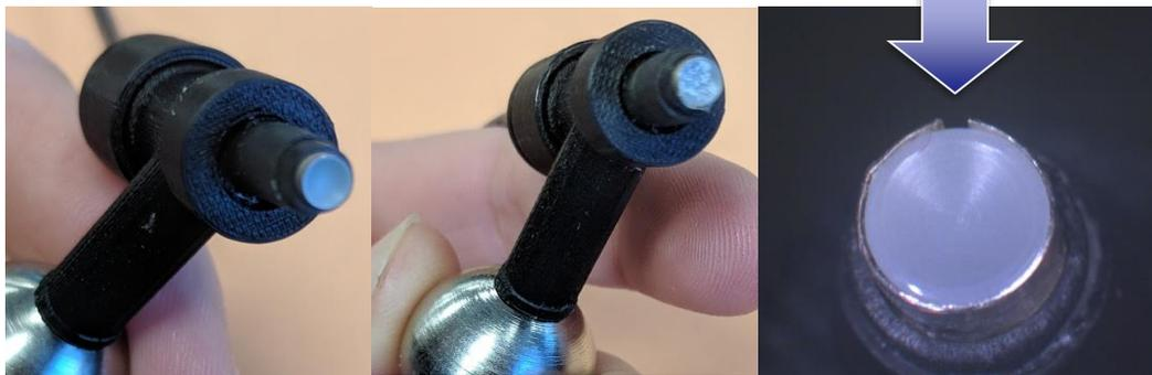
Figure 39 - a clean stimulator    Figure 40 - a dirty stimulator    Figure 41 - a stimulator that has been damaged during cleaning
