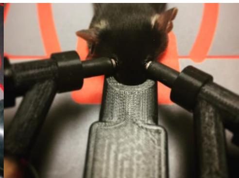
Figure 14 - The TOUCH/TOUCH Setup with gas nose cone
