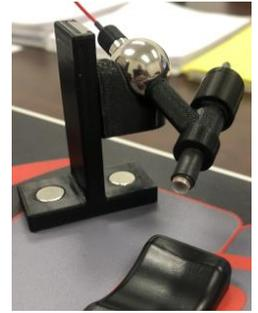
Figure 9 - T-bar increasing the height of the electrode
